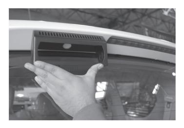
STEP 1. Place the ZROADZ LED Housing on the rear spoiler and mark the pre-determined (2) slots and (1) thru hole.
