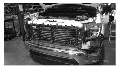
4. Remove the grille from the vehicle and set on a protected work surface.
