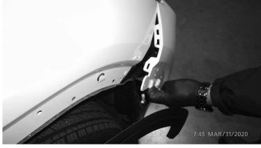
3.Remove the bolts retaining the grille to the core support under the headlight.
