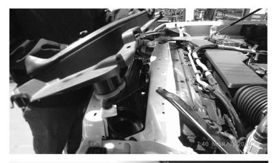
2.Remove the fender flares and pull the front facia away from the fender on both sides of the vehicle.
