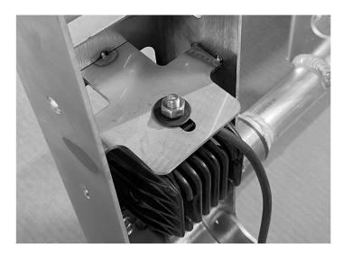
8. install (4) 2" LED lights into legs as shown using 8mm x 25mm hex bolt, flat washer and lock washer.
