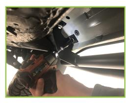
4) Using (8) M8 bolts for each side and the same mounting points as before secure the ZROADZ Side Step onto the underside of the truck.
