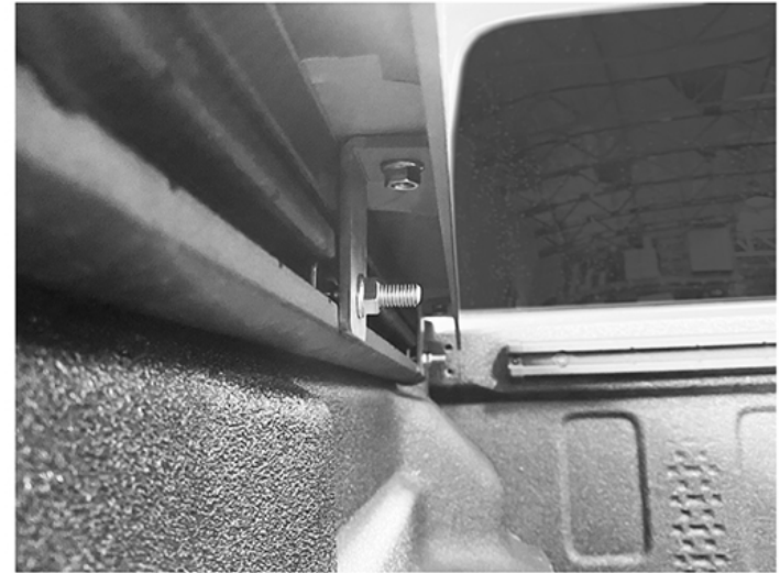
13. Install rack to vehicle and attach supplied track brackets as shown. Use (6) track inserts and hardware included with bracket components.
