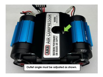
7.2. Install (1) JIC-4 to 1/4" NPT Elbow Fitting into the compressor's outlet port, applying Teflon tape or thread sealant to the NPT threads, and orient fitting downwards, as shown. Then, install the Stainless Steel Braided Air Hose onto the JIC-4 fitting. The Elbow Fitting and Braided Hose can both be tightened with a [9/16"] Open-Ended Wrench.
