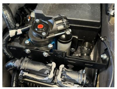
8.4. Using (2) [10mm] open-ended wrenches on both sides, proceed to fully tighten all 4 bolts securing the Compressor to the bracket, as shown.
