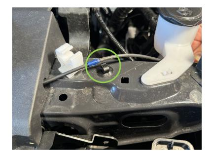
10.3. Before mounting the bracket, install the other end of the Stainless Steel Braided Air Hose to the JIC fitting on the Manifold, or Brass Bulkhead. Tighten with a [9/16"] Open-Ended Wrench.
