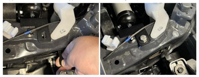
10.5. Install (2) M6 X 18mm Socket Cap Screws [5mm] with (2) M6 Oversized Washers into the Twin Compressor's threaded holes, joining the Manifold Bracket to the Compressor Bracket, as shown. For the ARB Single Compressor, install these screws using (2) M6 Flange Lock Nuts [10mm] on the backside of the Compressor Bracket.
