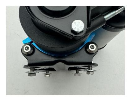
8.3. Pick up the compressor and tilt it so that all 4 washers contact the bolt heads, then, carefully feed the bolt heads and washers through the keyhole slots of the Compressor Bracket and slide the compressor down into place.
