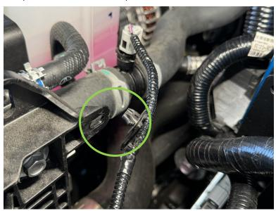
10.2. Pull hood-latch cable out from under clip, as shown.
