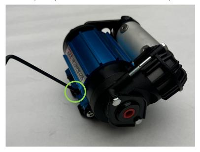
8.2. Using (4) M6 X 14mm Hex Bolts, (4) M6 Oversized Washers, and (4) M6 Flange Lock Nuts, partially thread the Nuts onto the Bolts inside the Compressor's mounting slots, with the bolt heads and washers on the bottom side, as shown.
