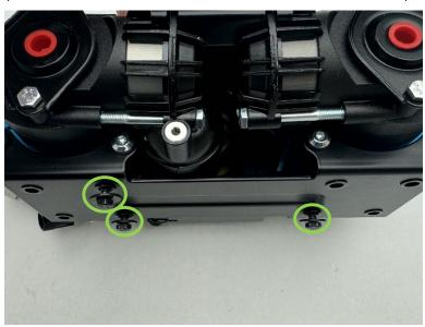
7.5. Pick up the compressor and tilt it so that all 3 washers contact the bolt heads, then, carefully feed the bolt heads and washers through the keyhole slots of the Compressor Bracket and slide the compressor down into place.
