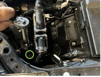
3.2. Install replacement bracket, Reinstall (1) factory bolt [10mm], (2) screws [8mm], and (1) nut [10mm].
